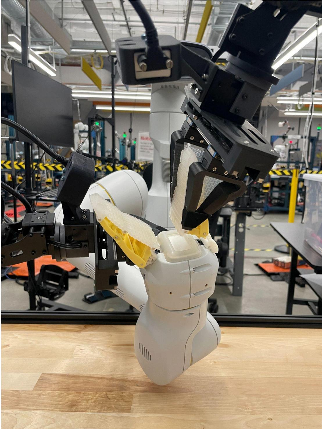
Step 5 [IMPORTANT]: Move the left arm as an “observer”, so the slot is inside the wrist camera’s view.
