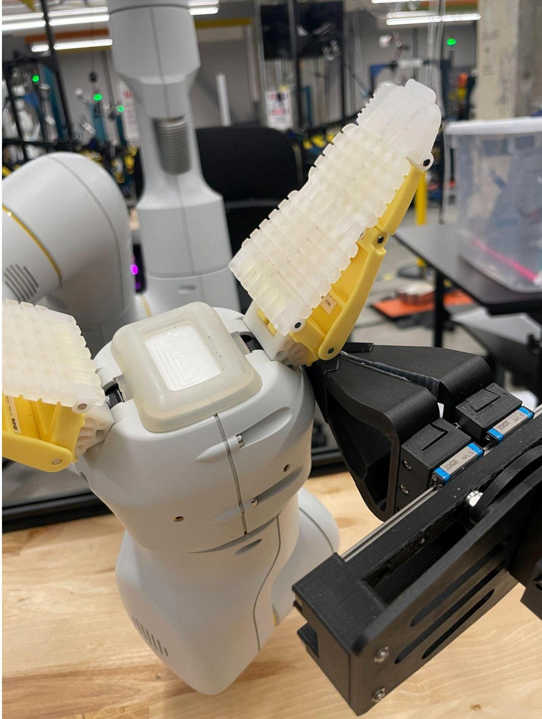
Step 2: grasp the MobileRobot finger tip with the left gripper, then use the right gripper to push out the finger.
