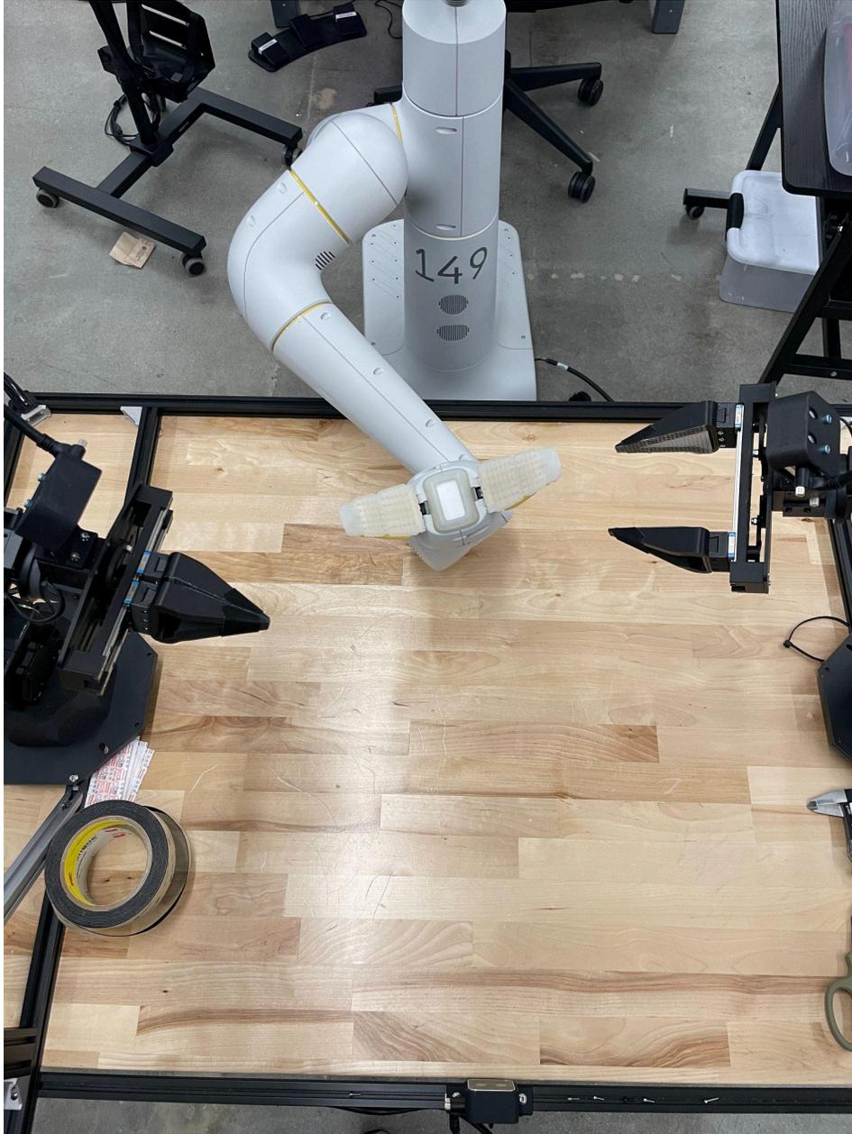
The MobileRobot robot should have its arm stretched out into the table. It should also be centered left-right with  $\pm 10$ cm (left image). The wrist of the MobileRobot should be slightly tilted (right image) to make insertion easier.
