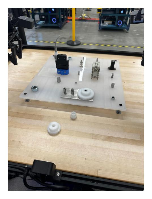
2. Using the **right arm only** pick up the middle size gear and put it on the middle peg. Note: the gears must be meshing so that both gears are sitting flat against the metal plate (as in the image below).
